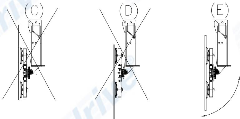
Check that all suckers on the surface are clean and have full contact and, if necessary, press on or align a sucker that is not making contact until it is in the correct position. If this is not done, a vacuum cannot build up and the VSG 6000 K MH can therefore not lift the material. Set the suction switch to the ON position using the remote control.
