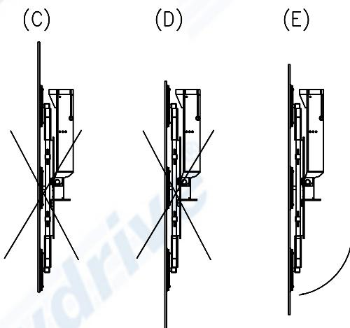
Check that all suckers on the surface are clean and have full contact and, if necessary, press on or align a sucker that is not making contact until it is in the correct position. If this is not done, a vacuum cannot build up and the VSG 4500 K MH can therefore not lift the material. Set the suction/release valves to the suction position using the remote control.
